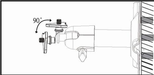
Loosen up the Thumb screw.
